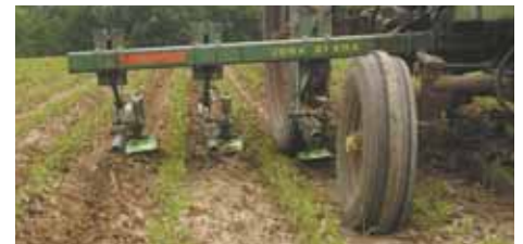
Flow-Shields can also be used for depth control, eliminating gauge wheels on each row. The extra down pressure on the Flow-Shields helps crush dirt clumps.
