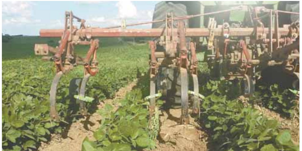
Flow shields are normally installed flat and can be adjusted to be angled toward or away from the row (as in this picture) to control the flow of more or less dirt into the row area.
