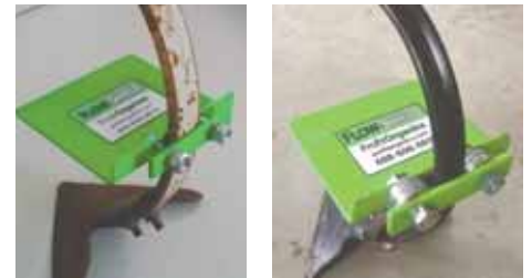
Flow-Shields simply bolt to cultivator shanks with no modification. Washers are used as spacers to firmly attach them to S-tine shanks.
