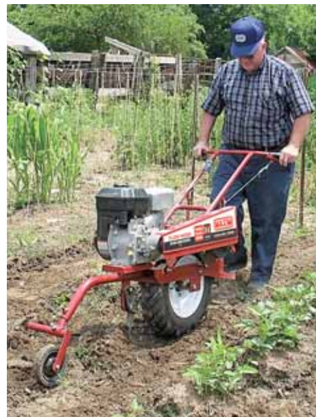
One-wheeled Plow Hoss is powered by a 127cc Briggs & Stratton engine. It comes with interchangeable accessories including a turn shovel, 12-in. sweep, and furrower.
