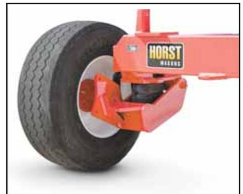
**Shock absorber blocks mount on steel cases that float on pivot pins, allowing each wheel to respond independently.**
