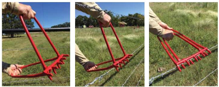
Hinged tool has 2 handles, both fitted with rows of interlapping teeth that form a "jaw" over wire. Operator pushes top half of tool down through bottom half to crimp the wire, then raises it back up to release wire. Wire Tight takes up 6 in. of slack with every "bite", which is why it works without breaking your old wire.
