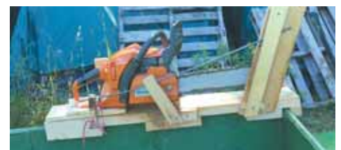
“Trigger rod” revs up chainsaw. It consists of a short rod that runs through chainsaw handle and under the trigger, and a longer “spring-loaded” rod that runs alongside chainsaw bar.
