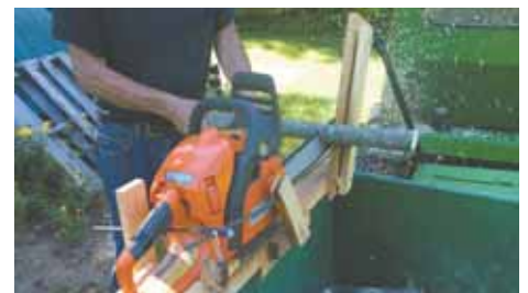
Wooden chainsaw holder is fitted with brackets that fit onto side of yard trailer. As Clark pushes tree limbs down on top of chainsaw bar, the cut piece falls into trailer.
