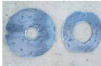
These two plates are used to mount the big flotation tires up front. Forde used a truck rim to make a “triple clamp” with welded-on bracing.
