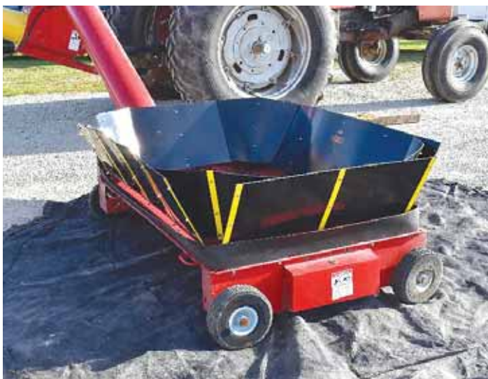
Extension kit bolts together using 8 spring-loaded plastic panels. The extra capacity allows grain trucks to unload faster and reduces unloading loss.
