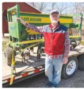
fields and get through small gates. Three rows of shanks are mounted on heavy-duty spring coils spaced 6 in. apart. The shanks are about 4 in. tall with a V-shape bottom that easily digs into existing pasture or tilled ground. Seed is dropped behind the shank at the depth set by gauge wheels on each side of the unit.
