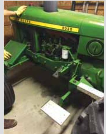
Homemade footpad and diamond plated step is safe and easy to use (above). Homemade brackets on other side of tractor support battery case and another step. Rinke improved the loader controls by installing a joystick control valve inside tractor's right fender.
