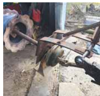
Pto-operated wire winder mounts on the reduction gear off a grain auger. An old wheel rim contains the wire.
