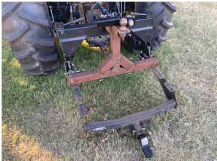
Home-built hitch bolts onto tractor's 3-pt. quick hitch and can move everything from trailers to wagons and implements.
