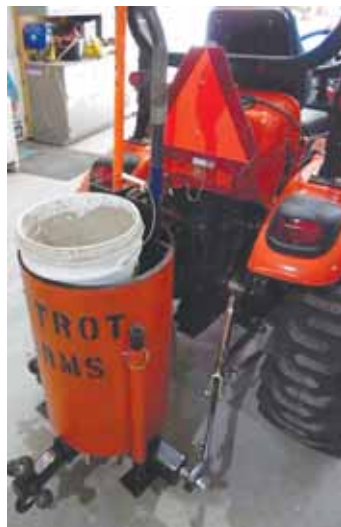
Sewer pipe welded to 3-pt. mounted bracket adds 240 lbs. of rear ballast.
