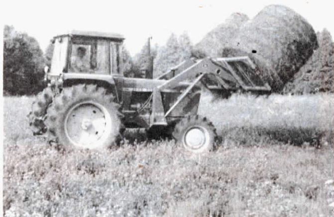
Bales can be stacked and retrieved two at a time with twin prongs.
