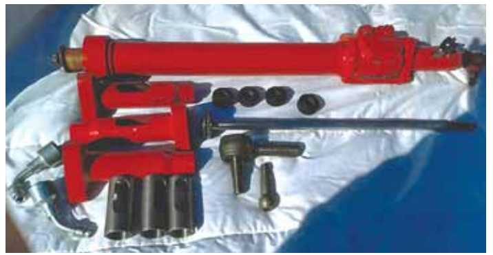
Hunter began repairing the Bendix steering assist units last year and has manufactured the parts that are no longer available. He’s had good luck making them like new again.
