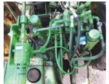
Bipes cut out part of tractor’s steering shaft to make room for an Eaton torque generator. New power steering unit was installed in existing hydraulic return line.
