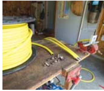
ColorStorm hose is available in up to a 330-ft. bulk reel (left). Hose Crimper Press, used to crimp fittings in place, comes with an L-wrench for manual tightening.
