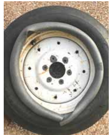
Tichavsky removed tire tube and wrapped foam pipe insulation around both sides of wheel rim. He then filled tire with air, injected tire slime, and trimmed off any excess insulation.
