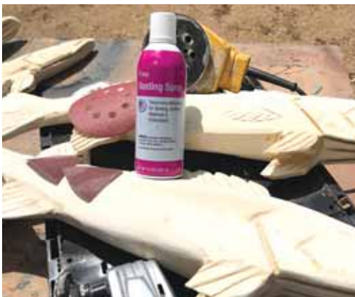
Basting spray is sprayed on sanding disc to stick it to the sanding pad. When disc wears out it can easily be pulled off.
