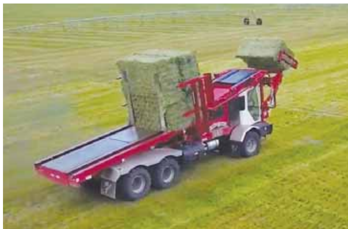
Justin Matlack says his Stinger Stacker 8500 is "bigger, better and faster" than the truck-mounted bale hauler introduced by his dad and uncle in 1999.
