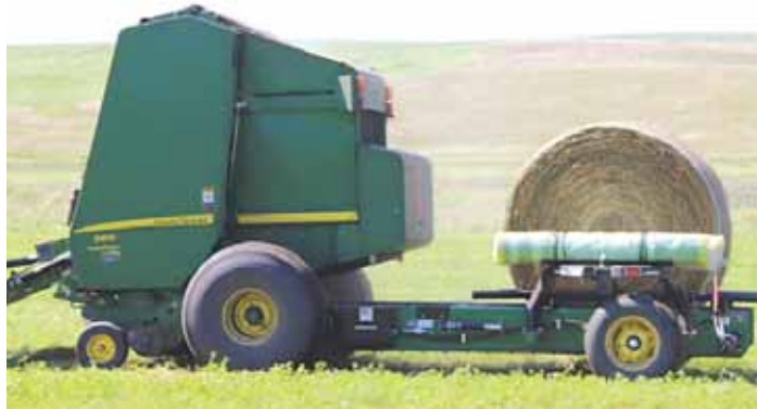
Lankota Bale Buggy carries a single bale until the second one drops, and then both are released to the ground. The design reduces crop damage and compaction.
