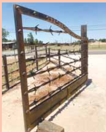
To make his popular barbed wire gates, Hedrick welds strands of 1-in. dia. "wire" with 3-in. long barbs to 4 by 4 metal posts.
