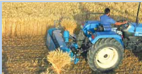
Pto-driven BCS Reaper Binder makes bundles of wheat and barley that can later be run through a plot thresher.
