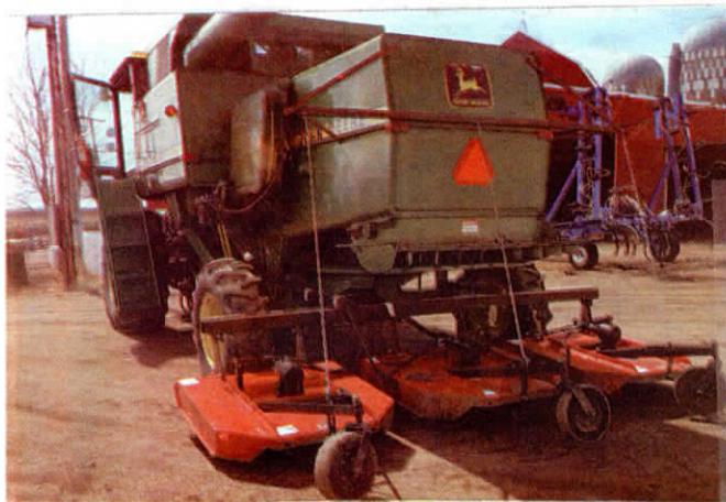
Combine stalk chopper consists of three hydraulic-powered mower decks suspended from bar that runs across rear of combine.
