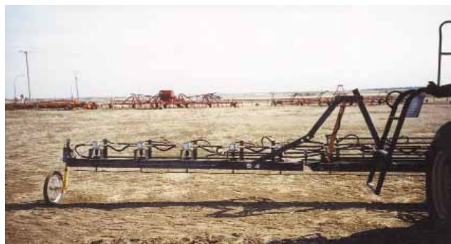
Cal Cowan converted a 1974 Gleaner combine into this self-propelled weed whacker.
