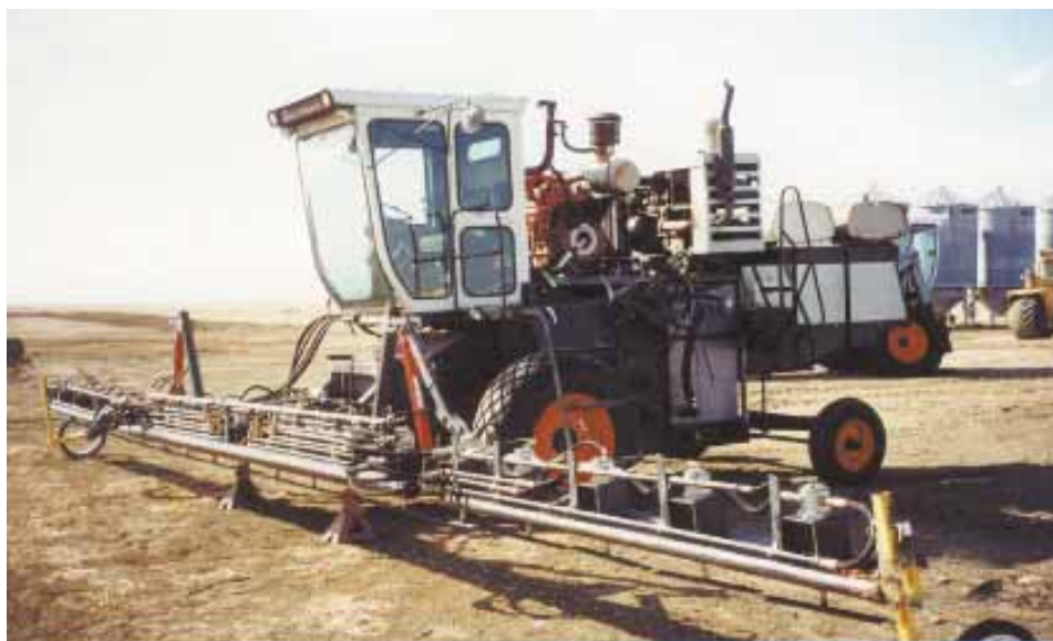
Cal Cowan converted a 1974 Gleaner combine into this self-propelled weed whacker.
