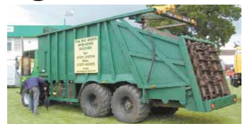
Four vertical spreader beaters mount on back of garbage truck. Truck's original hydraulic-operated ram pushes manure onto chain-driven slat floor in front of beaters.
