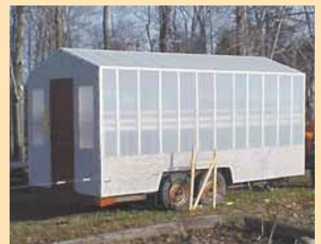
He cut a hole for a fan at one end and a doorway at the other end.
