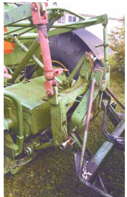
Back end of machine is fitted with a 3-pt. hitch, pto, and live hydraulics.
