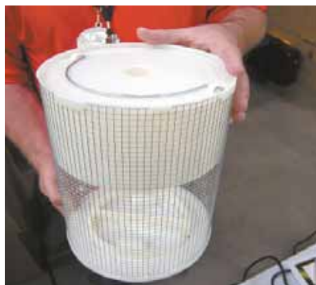
Mouse climbs up trap’s mesh sides and jumps through an entrance hole at top. To release the mouse you remove a plastic tray at bottom.
