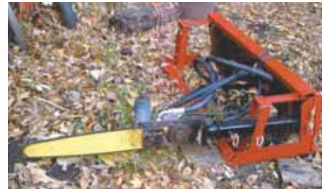
Skid loader-mounted chainsaw operates off the machine's hydraulics. It lets 93-year-old James Walsh still cut firewood now that it's difficult to handle a chainsaw manually.
