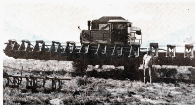
Morris built a second 40 ft. header, outfitted with twelve Hesston row units, for harvesting milo.
