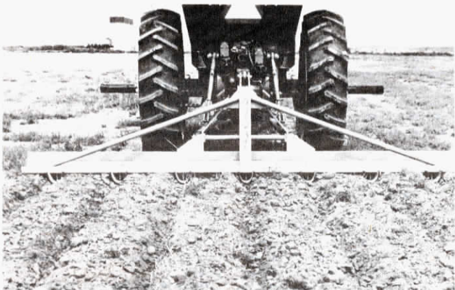
"Creasers" can be used to drain fields, to "pull" ditches, or as a bedding tool.
