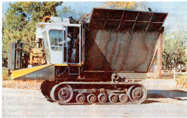
Tractor can also be fitted with a "lift-and-dump" grain hopper that raises up hydraulically to dump off to the side, emptying its 450-bu. load in less than a minute.
