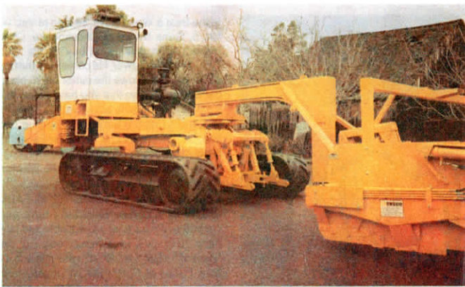
New rubber-tracked tractor can be equipped with a fifth-wheel hitch to pull heavy equipment such as laser scrapers or large tillage implements.
