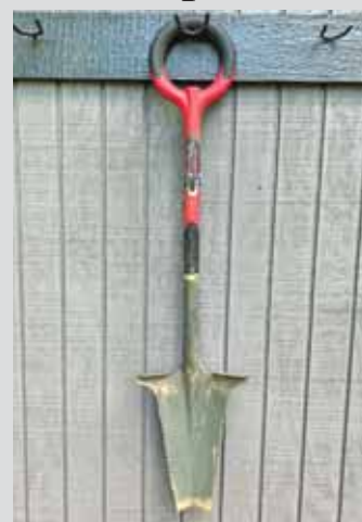
The Root Slayer has a carbon steel blade, ergonomic step and contoured grip O-ring handle.
