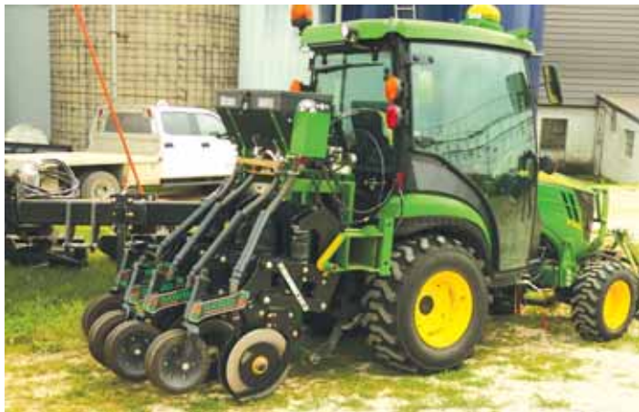
With DuoSeed units in the back and a mower deck on the front, cleaning up between rows and planting cover crops can be done in one pass.
