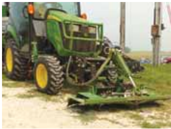
Recker modified the mower deck and 3-pt to front-mount the mower to his tractor.
