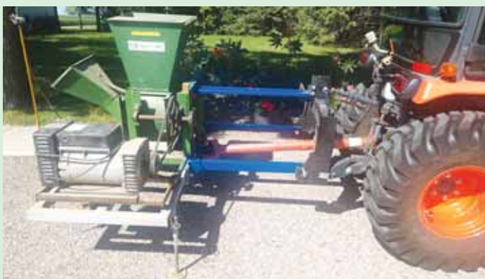
Negen's pto chipper/generator has an extended hitch and longer pto shaft.
