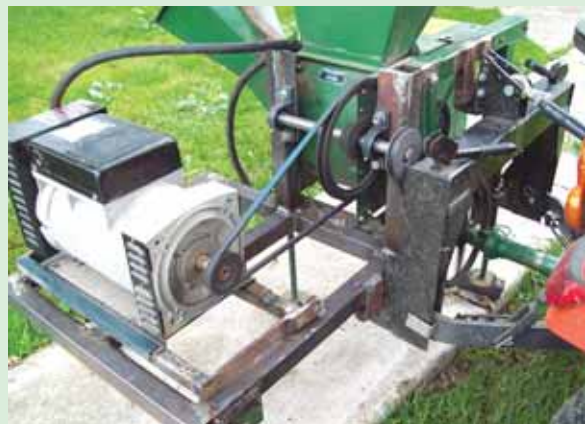
Detail shows the belt running both the chipper and generator.
