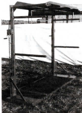
Bagging frame puts big square bales into tube-type silage bag and lets you stack bales 2-high.
