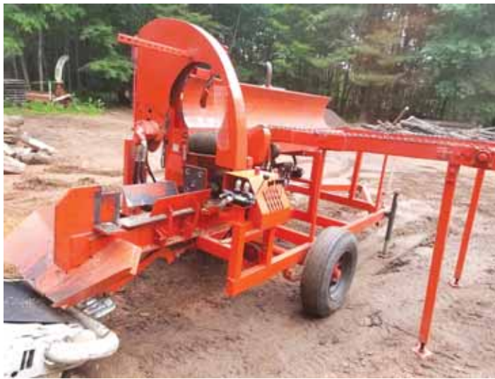
Carl Belohlavek built his firewood processor to handle up to 18-in. diameter logs using a 23 hp. Kubota motor.
