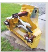
Steve Faber, Tiffin, Ohio: "To make a counterweight for my Deere 5085E tractor, I took the rear counterweight from a non-running forklift that I bought at an auction. I welded up brackets to fit and then drilled and tapped holes as needed. I made the mounting fit my quick hitch so I can quickly pick it up or drop it off. It weighs about 2,000 lbs. and is just about right on this tractor. I also plan to adapt the mast from the forklift to my tractor quick hitch."
