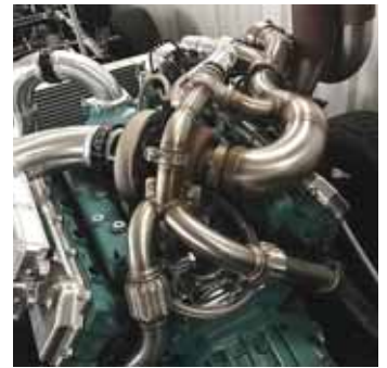
Art Martinez's 6.0L Powerstroke triple turbo engine puts out 650 hp., but he plans to boost that to over 1,000 hp. with modifications.
