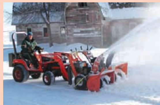
Tony Negen used a steel framework with tubing that slipped over loader forks to use two snow blowers bolted together and held down with ratchet straps to create a twin blower.
