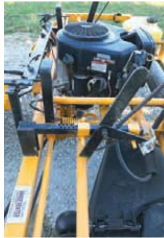
An 18-hp. Vanguard engine is used to power the two 46-in. mower decks.
