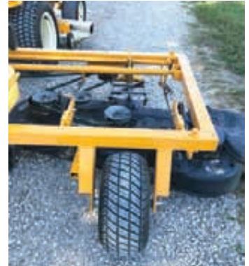
Vandeverter mounted double pulley drives on the engine driveshaft that run to upper pulleys and brackets, then to the decks.
