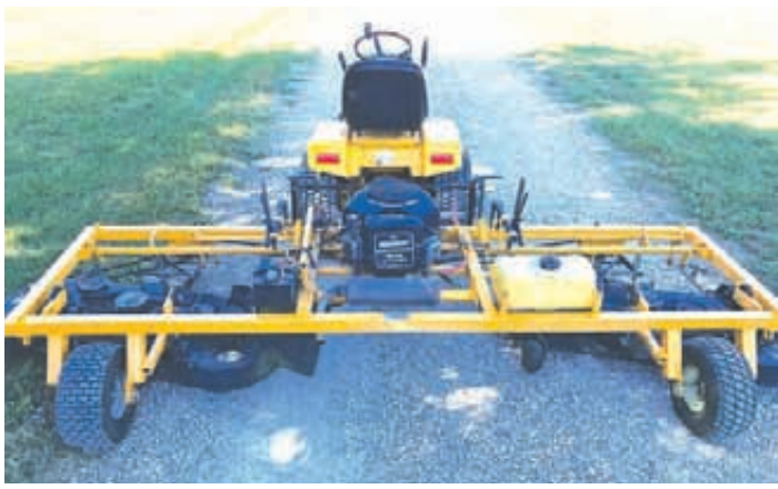
Two 46-in. mowers overlap the Cub Cadet's 48-in. deck by 4 in. and are mounted to a 9-ft. frame.
