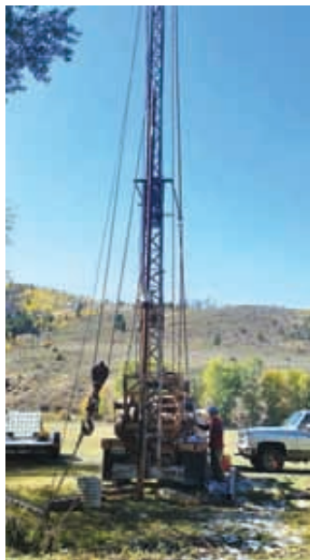
Cable drilling can be done year-round. The equipment costs less than rotary systems.
