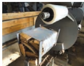
Lapp's firewood wrapper can be powered with compressed air or an electric motor and is operated by a foot pedal.
