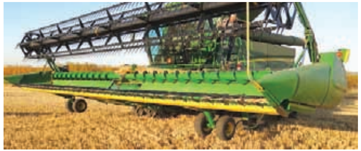
Cross auger attachment helps flow on flexible draper type swather and combine heads. It uses a flexible joint, does not need to be greased and has a patented stripper bar.
