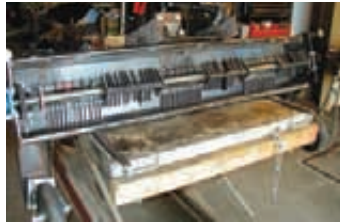
Dethatcher has swinging knife blades staggered every 1/2 in. on two rods that are 180 degrees apart.
