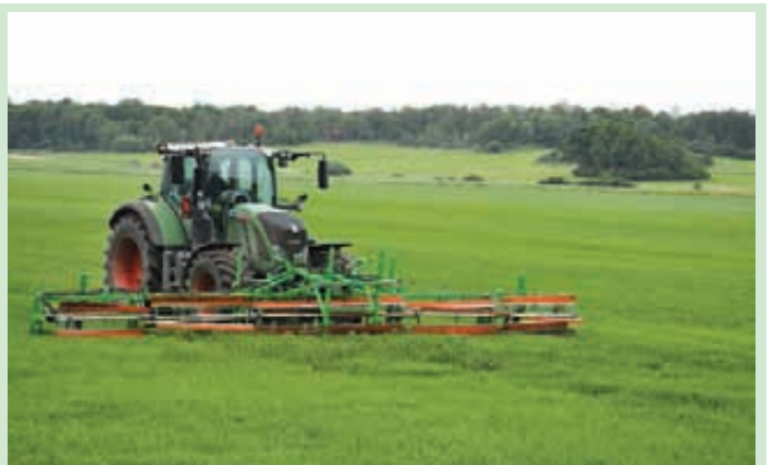
Combcut is available from 18 to 28 ft. working widths and can be front or rear mounted. It uses two double acting hydraulic outlets for brush/reel operation.
