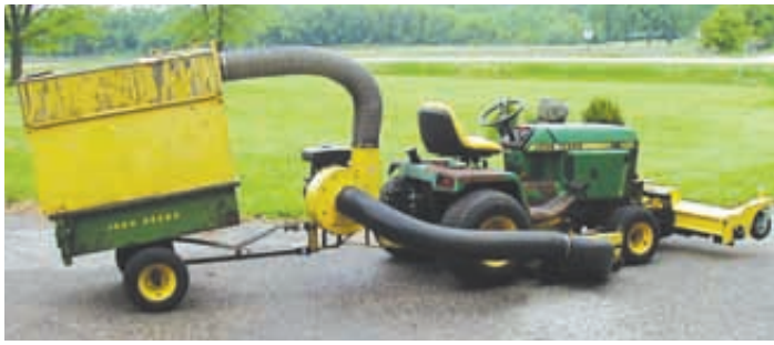
Tony Bunniss added a made-it-myself dethatcher to the front of his Deere riding mower and built a vacuum trailer to clear debris created by the dethatcher.
