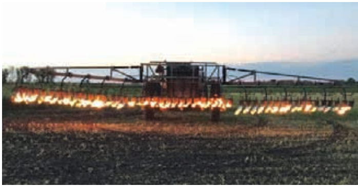
Sather's tow-behind flame weeder is available from 16 to 30 row widths and carries two 500 gal. propane tanks.
