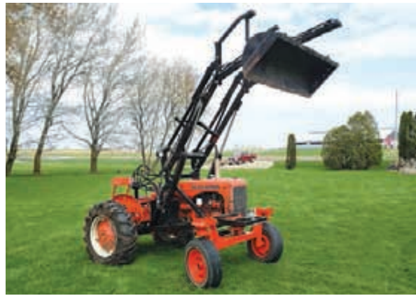
This modified Allis C has live hydraulics, a self-leveling loader and a wide front end with power steering.
