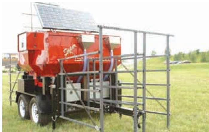
C-Lock’s SmartFeed system provides weight gain and water consumption data via Wi-Fi or cellular and has a solar power option.
