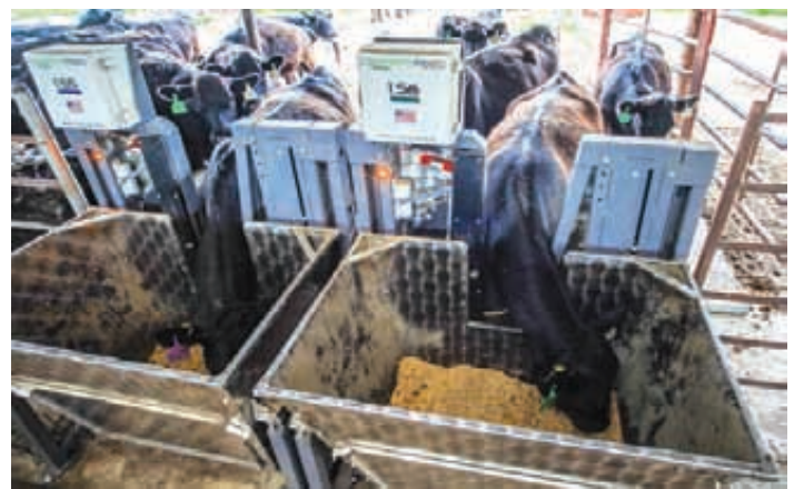
The SmartFeed system was used by one rancher to identify a bull that gained 6 lbs. per day and converted 3.52 lbs. of feed for each lb. of gain.
