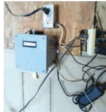
Actuator opens and closes the coop door (above). The system uses a low cost computer unit to operate and automate the door (below).
