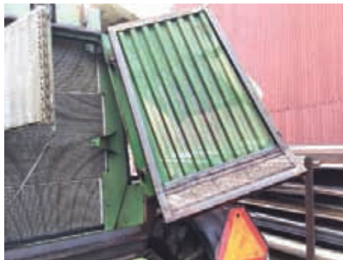
Varty made a frame to hinge the radiator and AC condenser on his Big M mower, making it easy to keep clean and avoid overheating.
