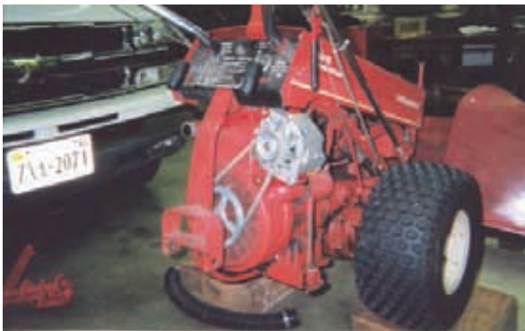
An alternator added to a Gravely 2-wheel tractor proved to be an economical solution to coil issues.
