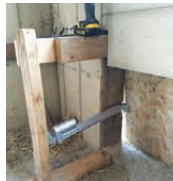
Actuator opens and closes the coop door (above). The system uses a low cost computer unit to operate and automate the door (below).
