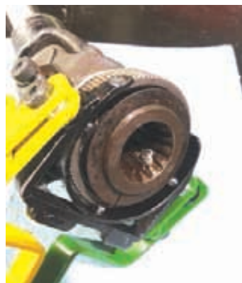
Bunniss made a pto tool to make it easier to change implements. His tool helps move the spring with less effort and better grip than doing it by hand.
