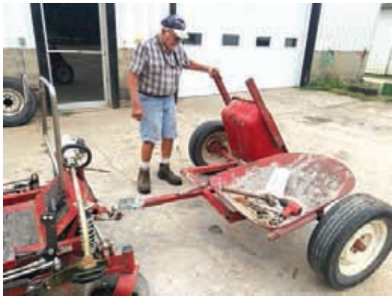
Hernke built a frame and fastened two wheelbarrows with piano hinges for a low impact hauler he moves with his zero-turn mower.
