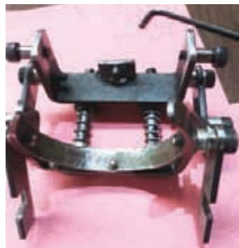
Bunniss made a pto tool to make it easier to change implements. His tool helps move the spring with less effort and better grip than doing it by hand.
