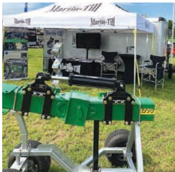
Transfer system can move weight from the center of a planter to the wings to relieve down pressure on the carrying wheels and help ensure uniform planting depth.
