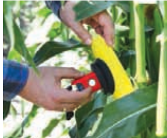
The SCiO Analyzer can read moisture levels from 80 percent down to 8 percent and sends info to a cell phone.
