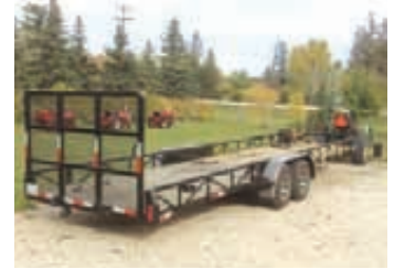
Friesen reinforced the joint sides, trailer extension, flooring and ramp of his 28-ft. trailer.
