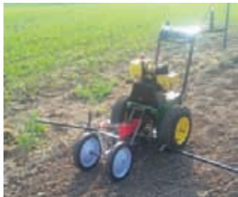
Bunniss fitted an EarthWay seeder to an old Deere snowblower to create an accurate self-propelled garden seeder.
