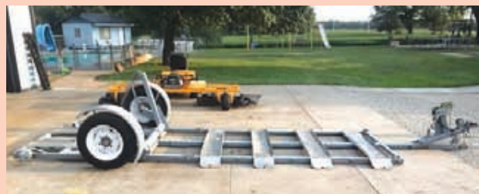
A winch cable is used to drop the trailer to the ground.
