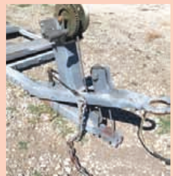
The cable runs through pulleys on the pintle hitch and trailer frame.
