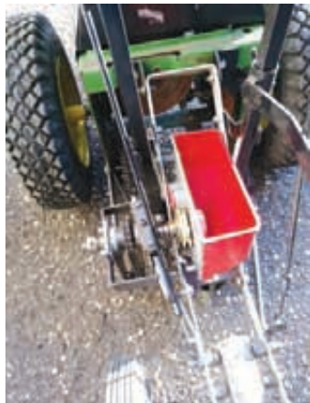
The custom seeder uses a positive drive system to mimic the EarthWay seeder ratio for seed spacing.
