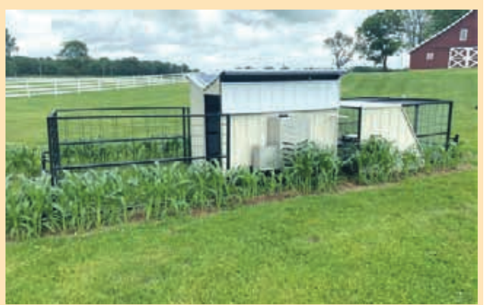
The solar powered barn and pen can move down a forage lane automatically providing grazing and no till without manually moving pens.
