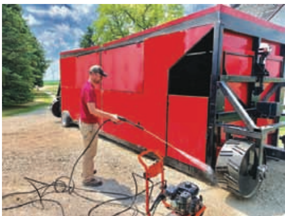
Two large steel wheels at each end of the barn move the unit forward and swivel as it’s moved on to the next forage strip.
