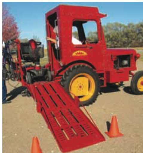
Harold Boquist modified his Empire 88 with a platform and ramp. The operator platform has two seats for him and his wife. There is even a rack on the back that can hold a walker.
