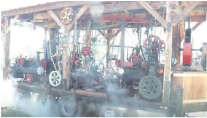
The trailer with 13 steam engines has 10 tires to carry the weight and is powered by an on-board boiler and separate steam tractor.
