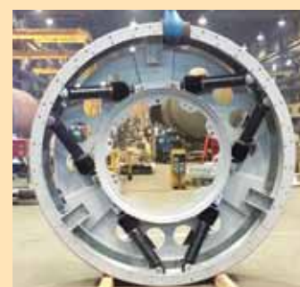
GACW’s new wheels are made of rigid steel and covered with polyurethane. Nitrogen cylinders inside the wheels provide flexibility.
