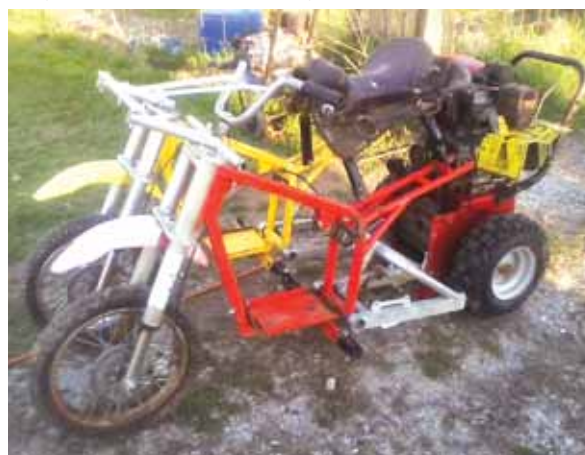
Smith built his hillbilly 4-wheeler from a snowblower, two old minibikes, and a pony saddle.
