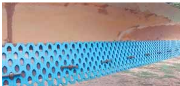
Sharq Edges blade system includes a mounting board that makes blade changes quick and easy.
