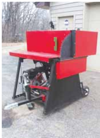
Bunniss's towable saw has a shielded blade and a platform that unlocks when a log is placed on it.
