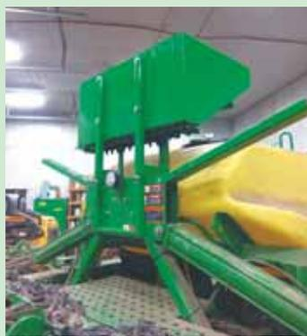
**Risch's seed box and brackets mount on a Deere air drill.**
