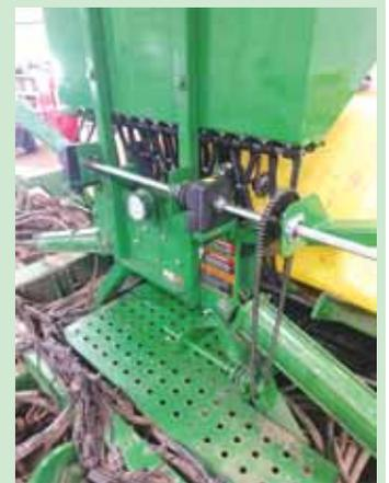
**Ground drive transfer with electric shutoffs.**
