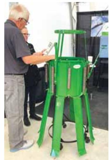
**The redesigned Agnew Spreader has a self-contained throat with an adjustable floor which is held closed with springs allowing for even grain distribution.**
