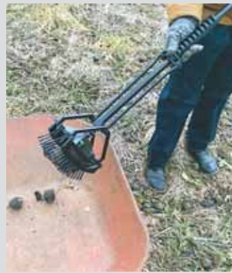
Stab-A-Nut has a handle that releases nuts into a pail or wheelbarrow.
