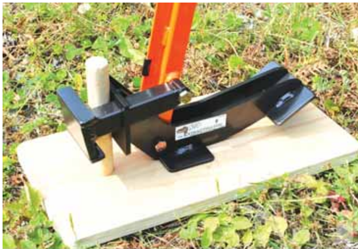
Extractigator is a hand-operated tree puller that's easy to use because its pivot point is close to the tree or plant.
