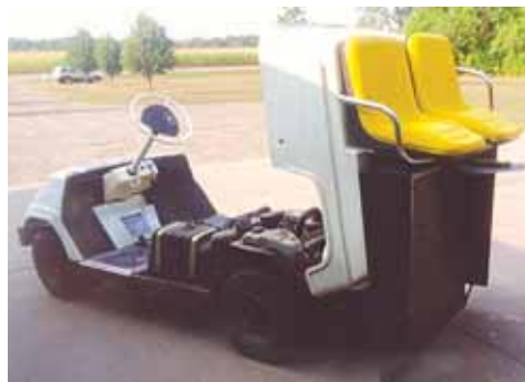
Adleman added a plywood box to his electric golf cart and added a steel hinge at the rear and mounted the box to it.
