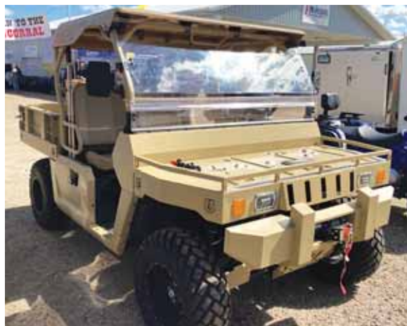
Warrior UTV is 6-in. wider than other UTVs and can seat three adults in the cab. It has a heavy-duty frame, 6-ply tires and a 500-lb. capacity electric lift box.
